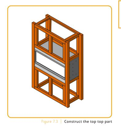
Make sure that the top part does not rest completely on the appliance and that a lintel is also installed at the desired height, so that the weight of the wall created does not end up on the appliance.
