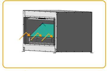
Figure 8.3 | Put the underside of the effect glass is the glass frame
