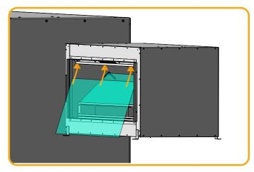
Figure 8.4 | Slide the front glass into the gap between the top profiles
