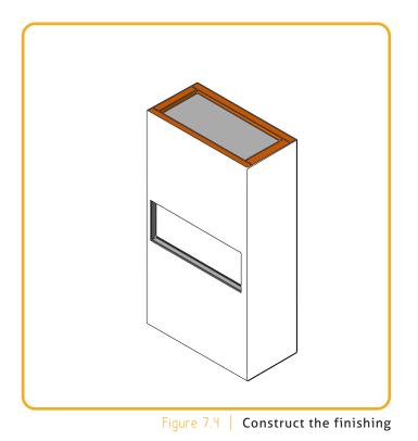
Make the cut-out in the plasterboard/finish board and install the fireplace, making sure that the plaster sealant edges align with the inside of the cut-out in the sheet.
