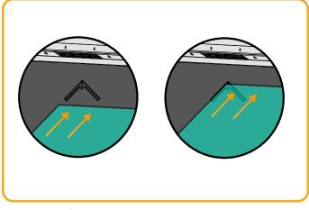
Figure 8.2 | Then slide the effect glass into the glass holders
