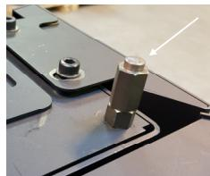
Adjusting the top plate is done by the 4 nuts located under the top plate.
