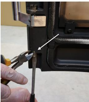
Remove the split and tighten the screw with a screw-driver (counterclockwise) depends on how much spring power you want in the handle.
