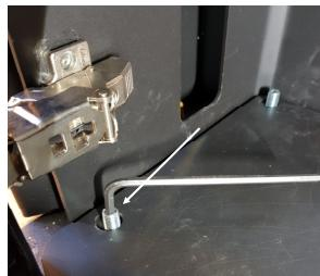
Adjusting the feet. One in each corner and one in the front of the firewood compartment.
